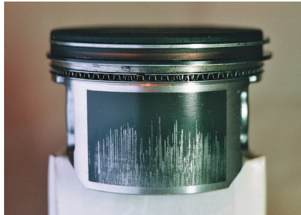
Figure 39 Piston Friction Reduction Coating Vertical Abrasion Pattern
